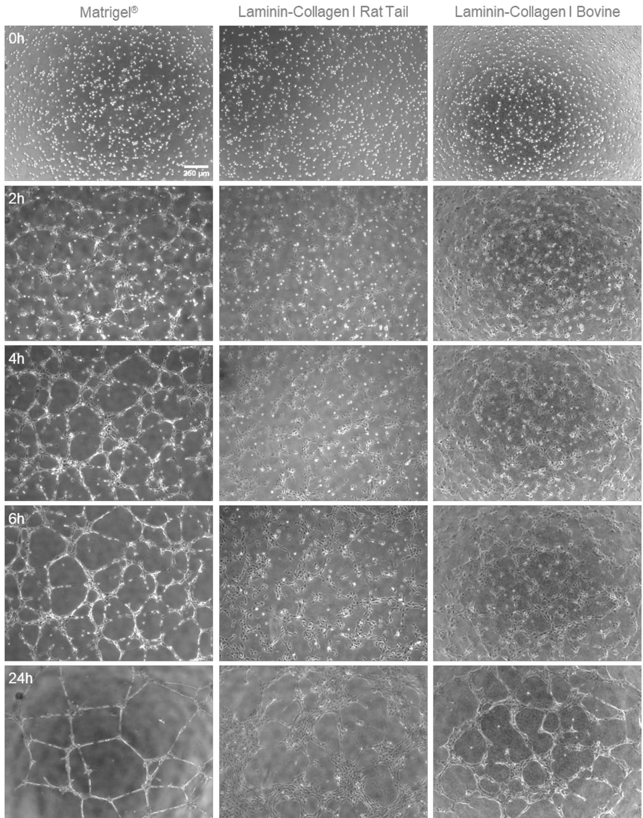
*Time lapse images of a tube formation assay using HUVECs in the  $\mu$ -Slide 15 Well 3D. Phase contrast microscopy with a 4x objective at 0 h, 2 h, 4 h, 6 h, and 24 h after cell seeding on Matrigel® (left), Laminin-Collagen I Rat Tail gel (middle) and Laminin-Collagen I Bovine gel (right).*
