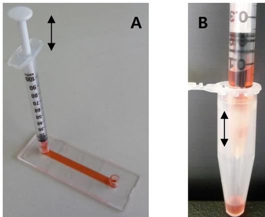
**Figure 3:** **A)** µ-Slide I<sup>0.4</sup> Luer filled by the pipette. Lyse cell layer in channel slide by moving the plunger up and down. **B)** Homogenize the cells with syringe and needle by moving the plunger up and down.
