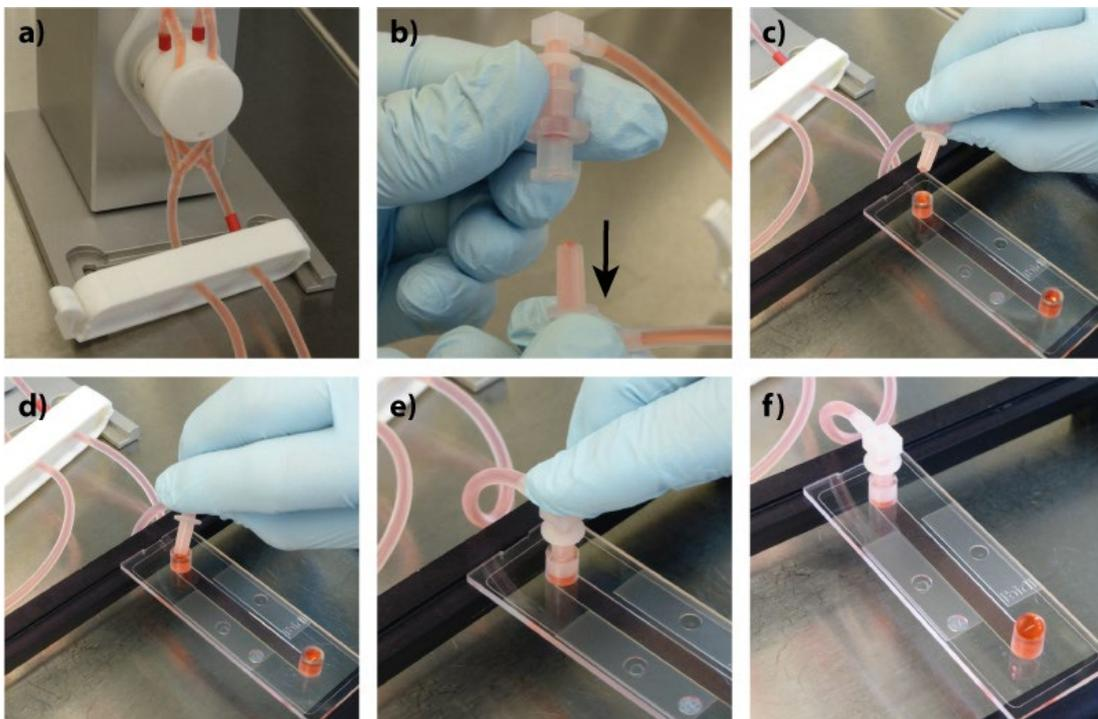
Figure 7-1: Connecting the  $\mu$ -Slide to the Perfusion Set (first adapter).
