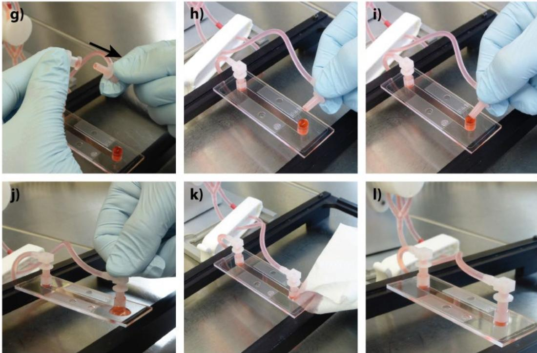
Figure 7-2: Connecting the  $\mu$ -Slide to the Perfusion Set (second adapter).
