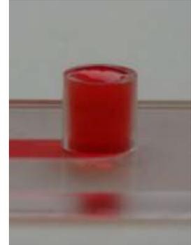
Figure 6: Luer port filled for connecting.
