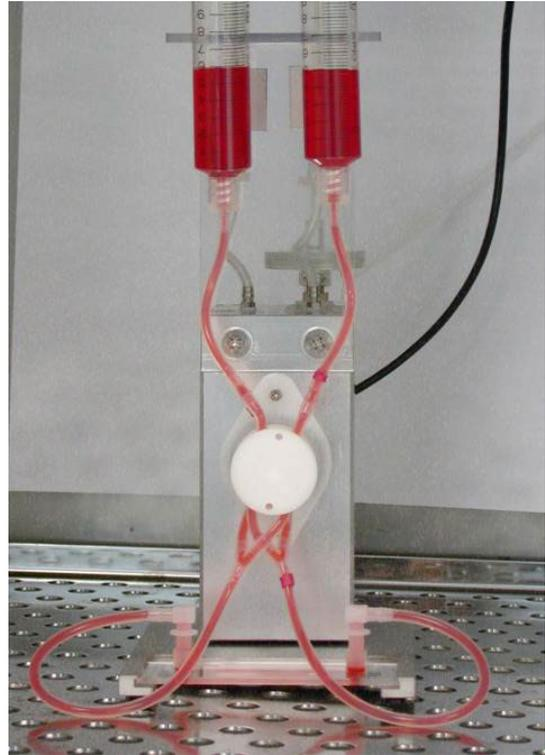
Figure 8: Fluidic unit with Perfusion Set and a  $\mu$ -Slide I Luer in the incubator.
