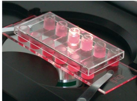
Besides the ibiTreat version (tissue culture-treated), the  $\mu$ -Slide VI<sup>0.4</sup> is available with different coatings (uncoated, Poly-L-Lysine, Collagen I, and Collagen IV). With the  $\mu$ -Slide VI<sup>0.5</sup> Glass Bottom, ibidi also provides a version with a glass coverslip bottom for special microscopy applications.
