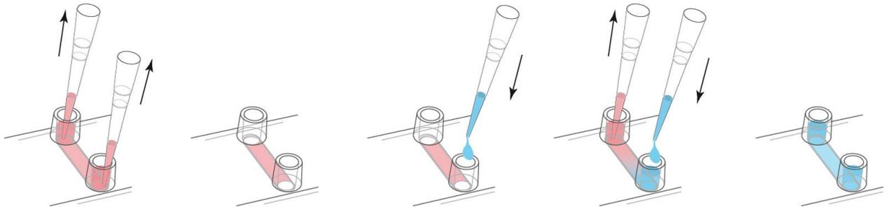
*Continuous exchange of medium with minimum 3 times the channel volume.*
