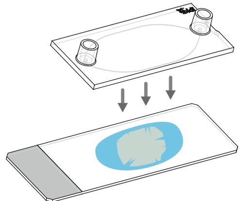
6. Fill the channel using a syringe or a pipet. Incline the slide and inject the liquid in an upwards motion so that air can escape above the liquid level. Optionally, connect Luer adapters and tubing for automated liquid exchange.
