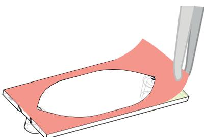
5. Mount microscope slide and sticky-Slide by pressing firmly with your fingers (use gloves) until both parts are completely sealed. Make sure the tissue section is aligned with the channel. For a better visualization of the tissue section, a dark background is beneficial.
