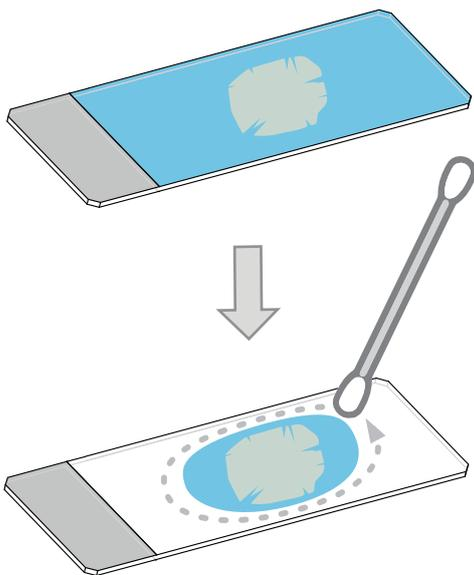
4. Remove the protection film from the sticky-Slide. First, scrape off a corner of the protection film using a scalpel or pointy tweezers. After that, grab this corner and remove the protection film.
