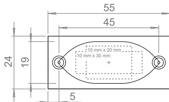
The sticky-Slide Tissue is made for tissue sections smaller than approx. 10 mm x 30 mm or 15 mm x 20 mm, respectively.
