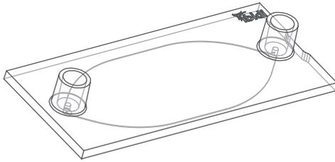
The sticky-Slide Tissue supports immunofluorescence and immunohistochemistry staining protocols of tissue sections on microscope glass slides.
