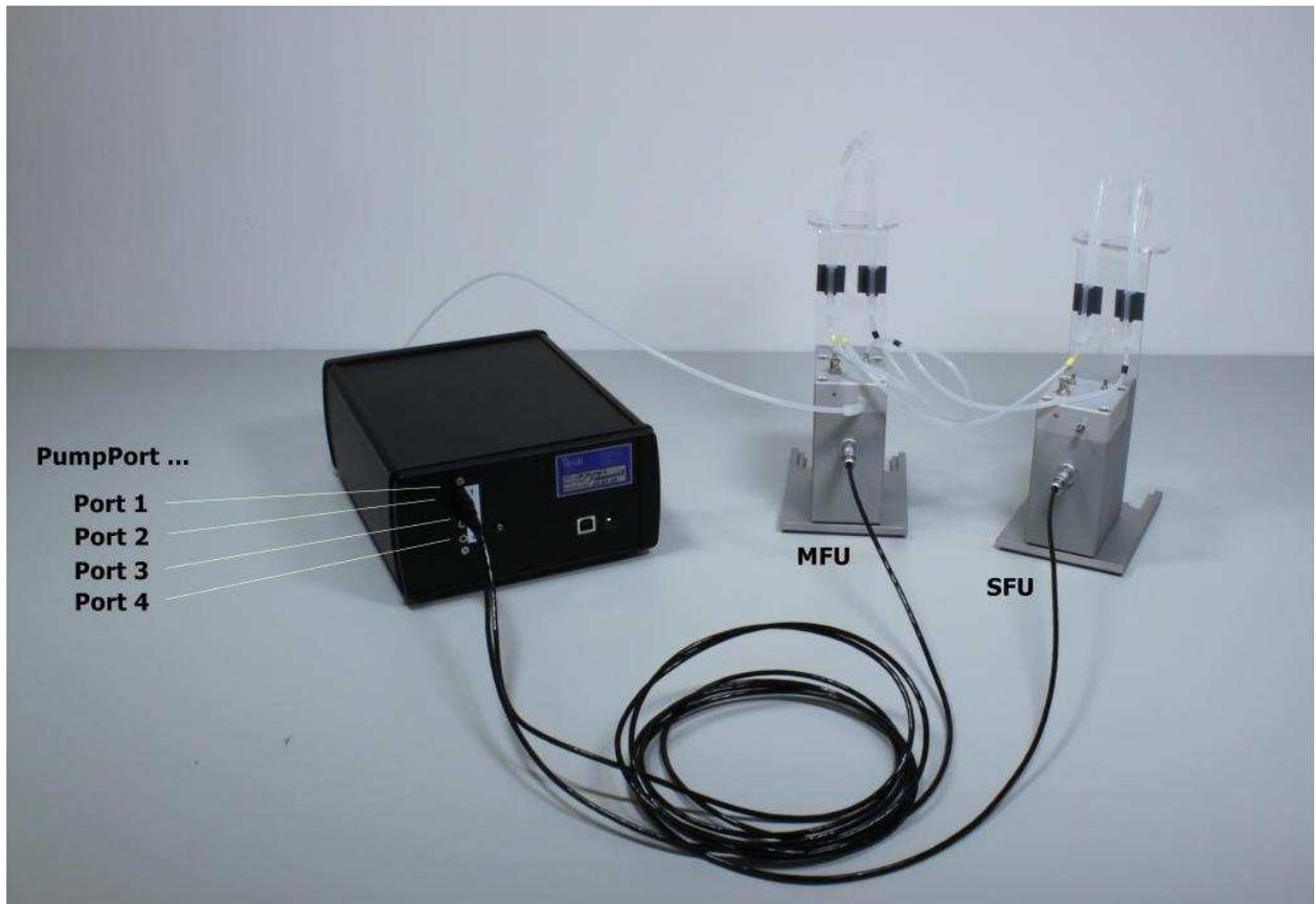
**Figure 3: Connected master (MFU) and slave Fluidic Unit (SFU)**
