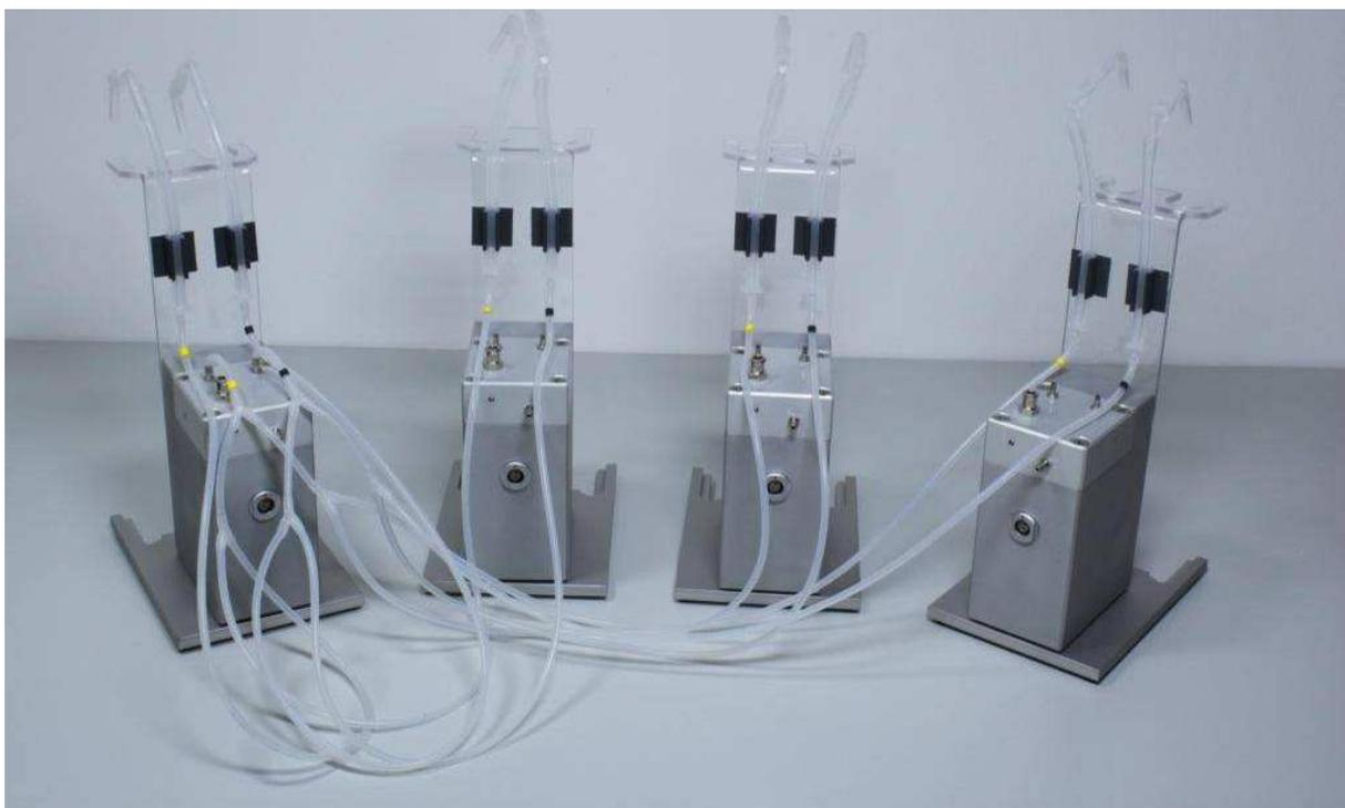
**Figure 5: Air pressure connection with a setup using 4 Fluidic Units**
