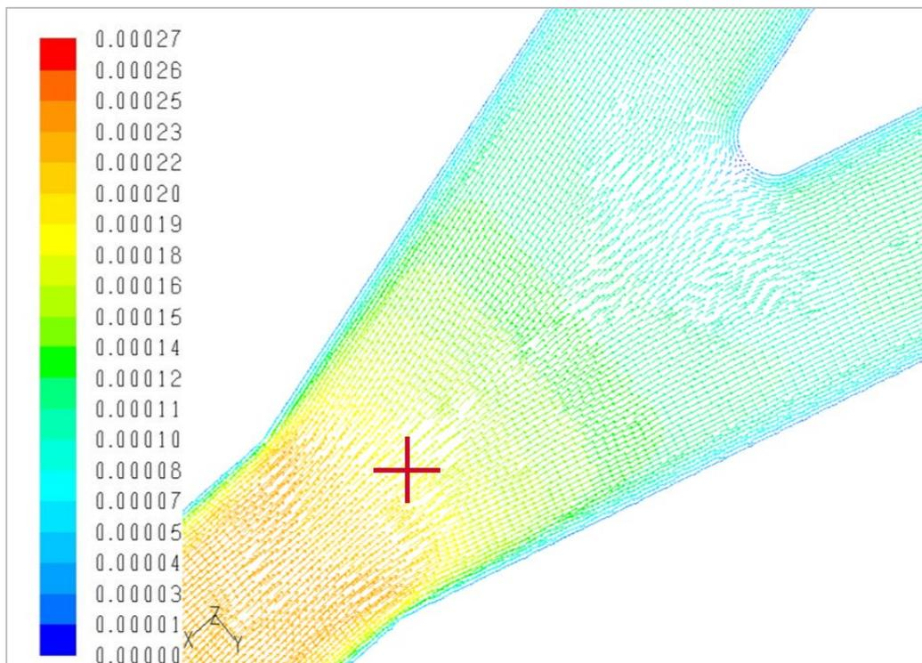
Figure 3: Calculated data for the 30° branching region. The arrows indicate the flow direction. The color scale gives the velocity [m/s]. The spot used in the calculation example is marked with a red cross.
