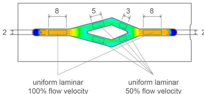
Figure 1: Bottom view of the  $\mu$ -Slide y-shaped. The dashed rectangles indicate zones of uniform laminar flow and, therefore, also uniform laminar shear stress. Measures in mm indicate the size of the zones.
