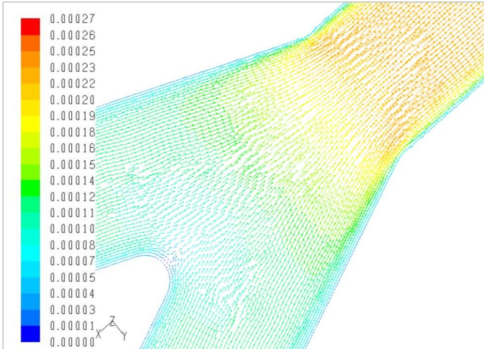
Figure 4: Calculated data for the 45° branching region. The arrows indicate the flow direction. The color scale gives the velocity [m/s].
