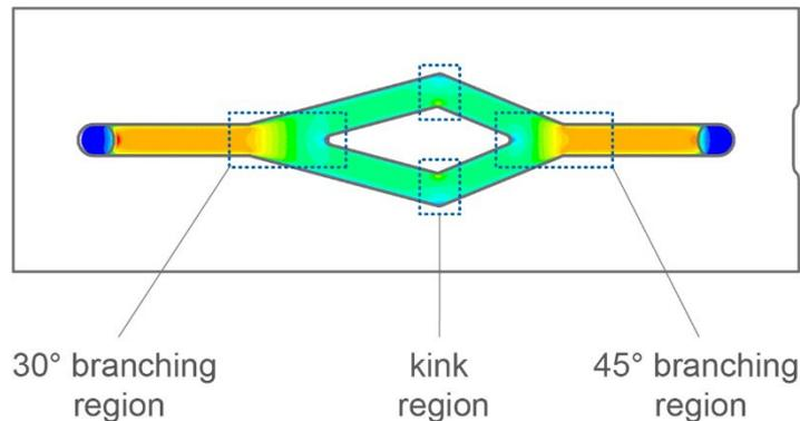
Figure 2: Bottom view of the  $\mu$ -Slide y-shaped. The dashed rectangles indicate zones of non-uniform laminar flow and, therefore, non-uniform laminar shear stress. The branching region on the left provides an opening angle of 30°. The branching region on the right provides a 45° opening angle.
